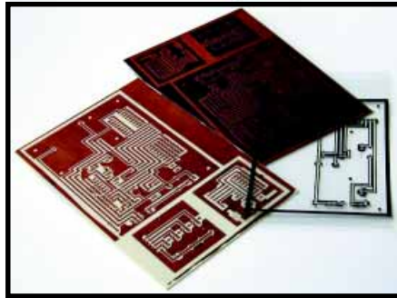
Photo 4 —From left to right, here's an etched PCB, PCB with developed resist before etching, and a mask on a transparency.
