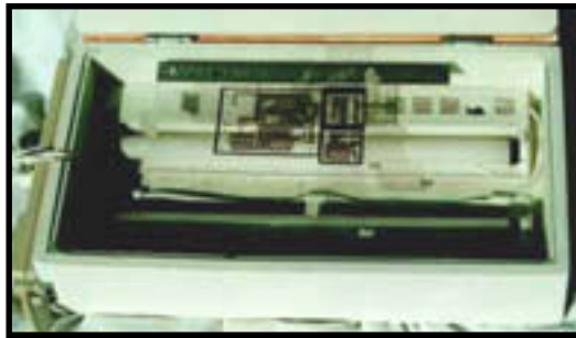
Photo 1—Check out the UV table with mask. You can see the UV lamps beneath the glass.
